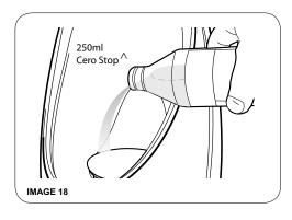
Pour 250 ml of IFO Cero Stop oil ^ into the urinal bowl and wait for the oil to fill the urinal cavity.
