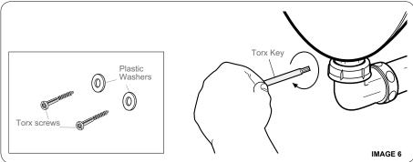
6. Fix torx crews to ensure the urinal is firmly fixed to the wall. **SEE IMAGE 6**
